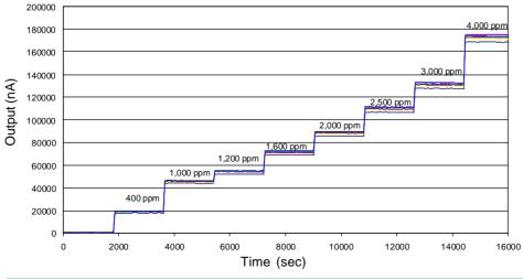
Figure 4 shows sensor output for increasing concentrations of CO to twice the specified overgas range. The data is derived from 8 sensors taken from a full production batch.
