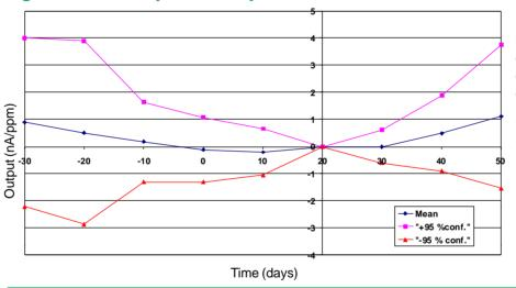
Figure 3 shows the variation in zero output caused by changes in temperature expressed as ppm gas equivalent.
