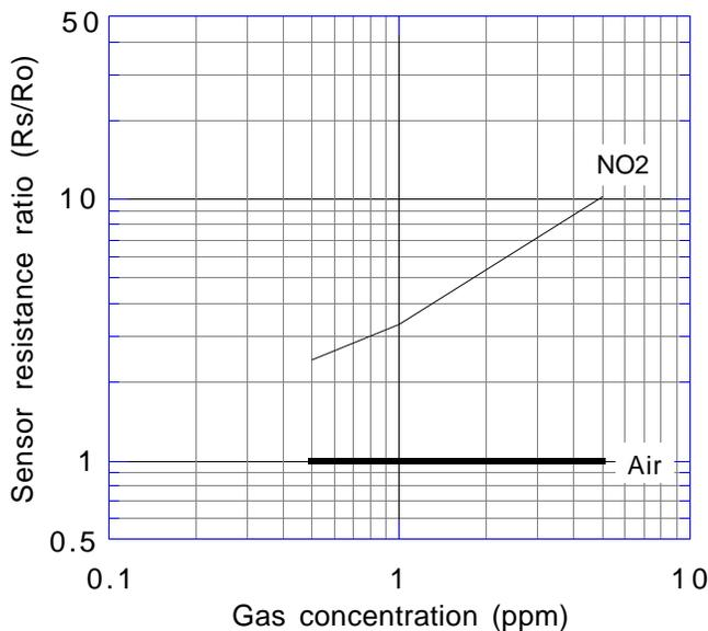
The figure below represents the typical response pattern of the TGS2106 when the atmosphere changes from clean air to the listed gas concentrations and then reverts back to clean air again.
