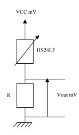
Vout (mV) =  $\frac{VCC (mV) * R (\Omega)}{R (\Omega) + HS24LF (\Omega)}$
