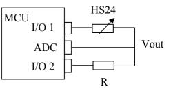
To prevent polarization of the sensor, resistive sensors use symmetrical AC excitation voltage with no DC bias. In this method, AC excitation is generated and managed by microcontroller I/O.
