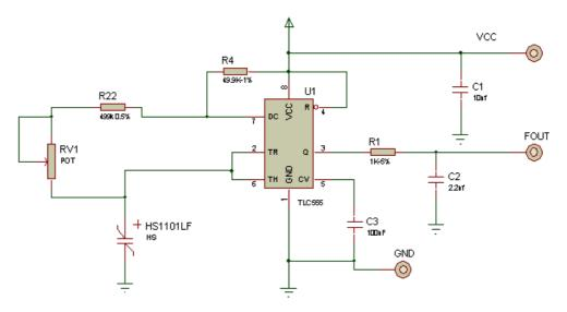
Note: R22=499k $\Omega$  / R4=49.9k $\Omega$  / R1=1 k $\Omega$  / RV1=50 k $\Omega$  potentiometer / C1=10nF / C2=2.2nF / C3=100nF
