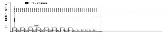
Fig. 6e: RESET sequence (21 bit).
