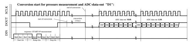
Fig. 6a: D1 ACQUISITION sequence.
