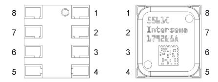
Fig. 2: Pin configuration of MS5561
