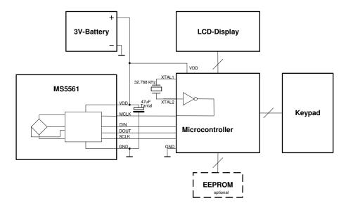
Figure 7: Demonstration of MS5561 in a mobile altimeter.
