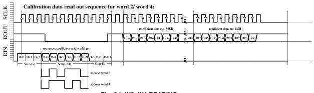
Fig. 6d: W2, W4 READING sequence.
