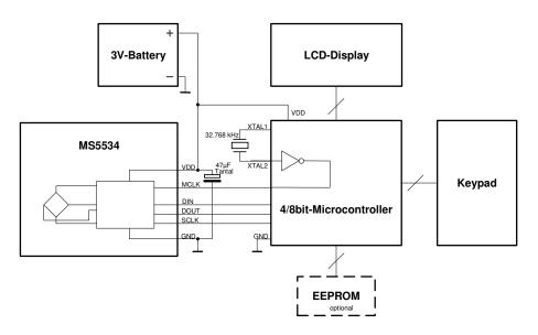
Figure 7: Demonstration of MS5534C in a mobile altimeter.
