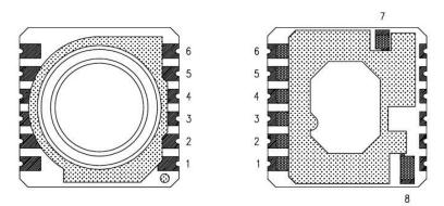
Fig. 2: Pin configuration of MS5534CM.
