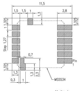
Pad layout for bottom side of MS5534C soldered onto printed circuit board
