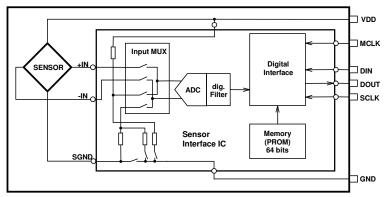
Fig. 1: Block diagram MS5534C.
