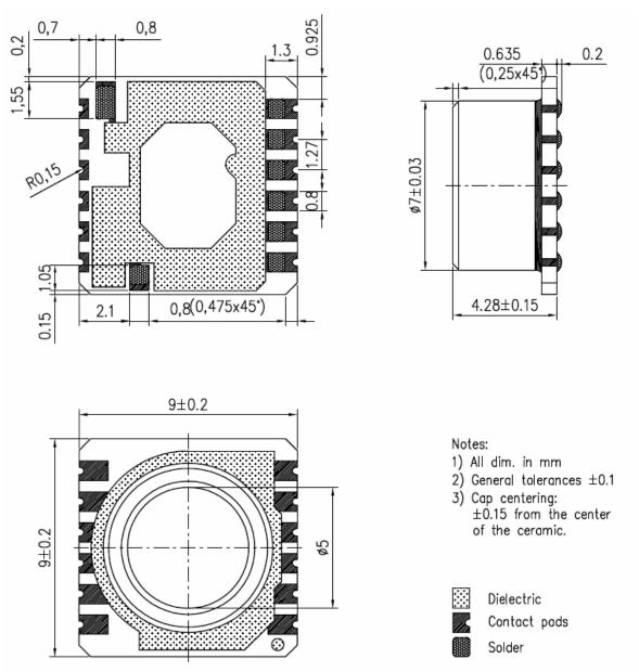
Fig. 9: Device package outlines of MS5534CM.
